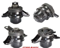
12305-B1021 TOYOTA PASSO KGC10 2004-2010, DAIHATSU BOON M300 2004-2010, DAIHATSU SIRION M300 2004-2010 12305-B1020 ENGINE MOUNTING
